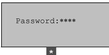
If the password is incorrect or when **\*** is pressed the device returns to standby mode.
